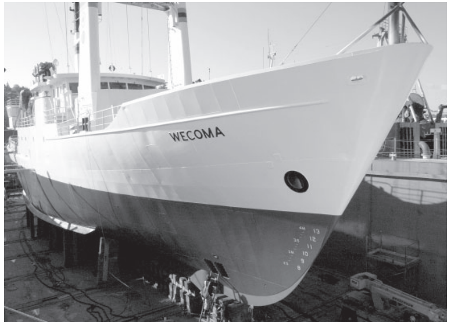
A shipyard worker inspects the bow thruster of the research vessel Wecoma, which has a new paint job and is nearly ready to leave the drydock.
