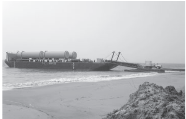
With the Beach Bear's ramp down, cargo is hauled off the barge toward the oil development site at Chayvo.
