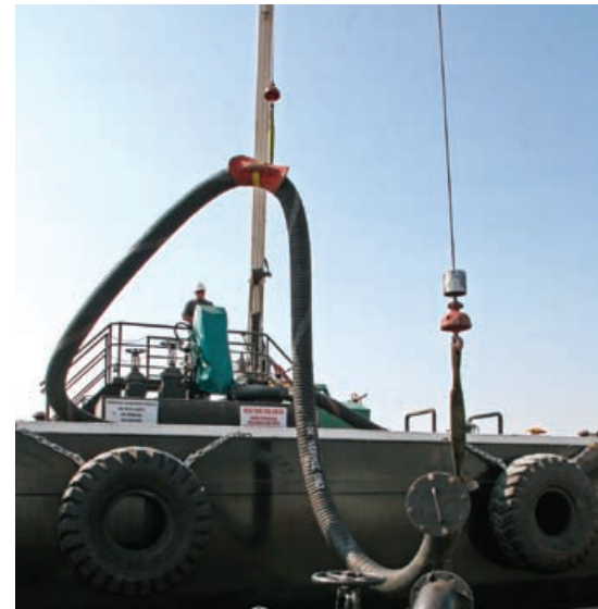
Joe Sasso uses the barge's crane to line up its product hose with a supply line at an oil terminal at the Port of Los Angeles.
