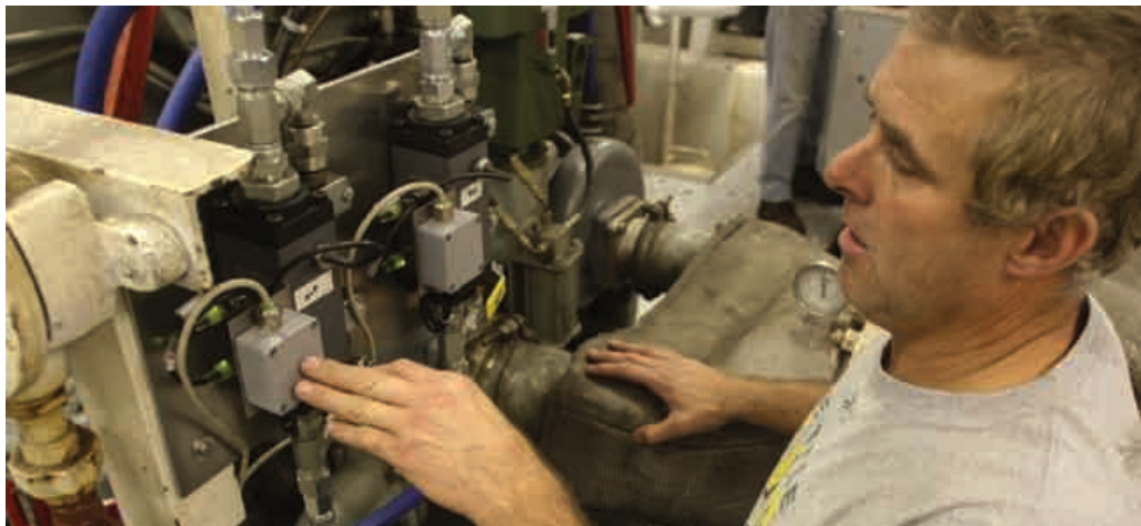
Engineer John Judd points to the flow detection devices on the fuel lines to one of the main engines. In the photo below, a display in the pilothouse of the Garth Foss keeps deck officers apprised of fuel consumption.
