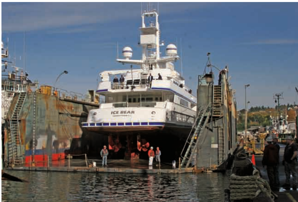
The Itasca , above, was drydocked at Foss Shipyard for five weeks, followed by the Ice Bear , shown in a drydock being nudged into Foss Shipyard. The drydock had been moved out of its berth into deeper water for the operation so it could be submerged enough to accommodate the Itasca .
