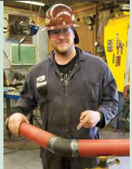
Foreman Chris Intagliata displays a high-quality “TIG” weld executed in the Seattle Pipe Shop.
