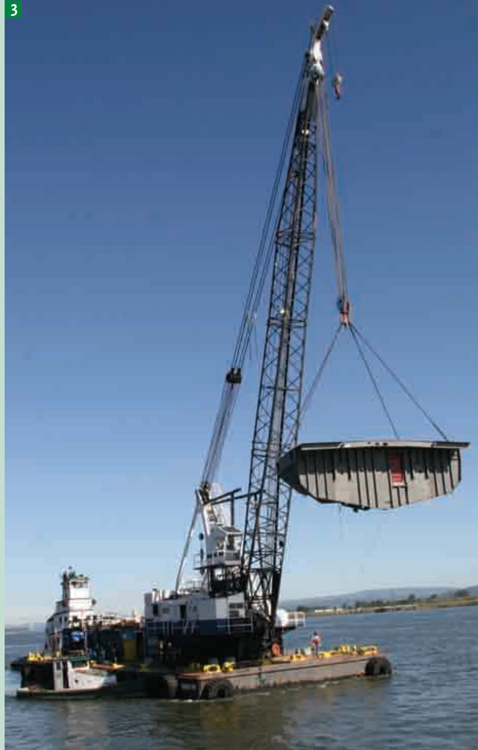
3 The distance is only a few hundred feet across the shipyard, but the easiest way to move the stern section is by water.
