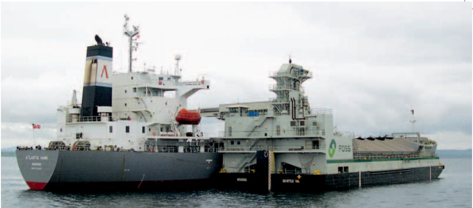
The Foss barge Noatak lightens ore to a ship near the Red Dog Mine port.
