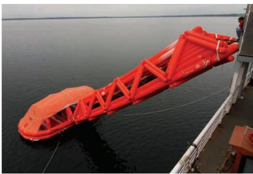
An evacuation slide is deployed during tests on the Alaska state ferry Aurora.
