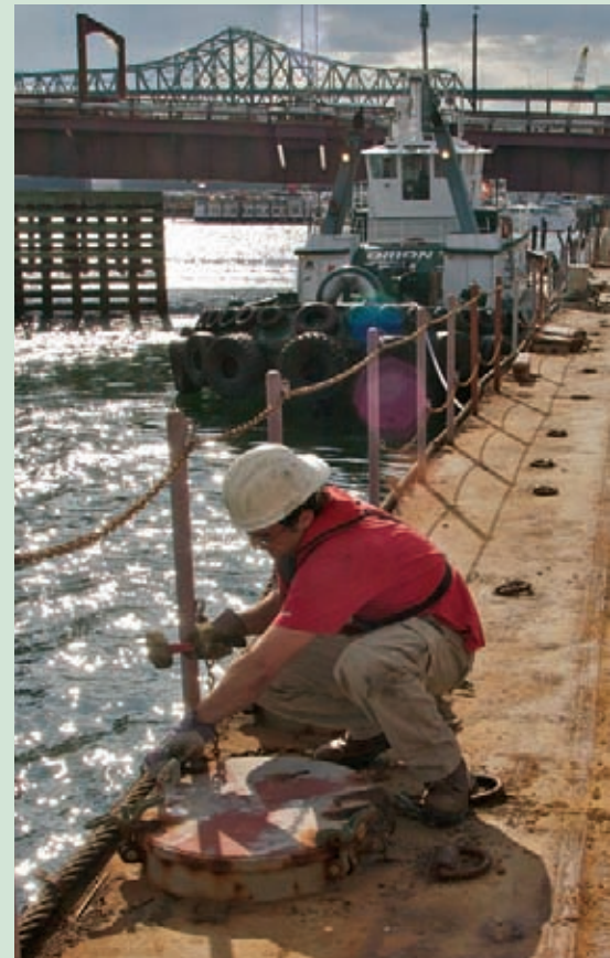
Arthur Ladd dogs down a hatch on the Chem Caribe in preparation for the sea voyage.
