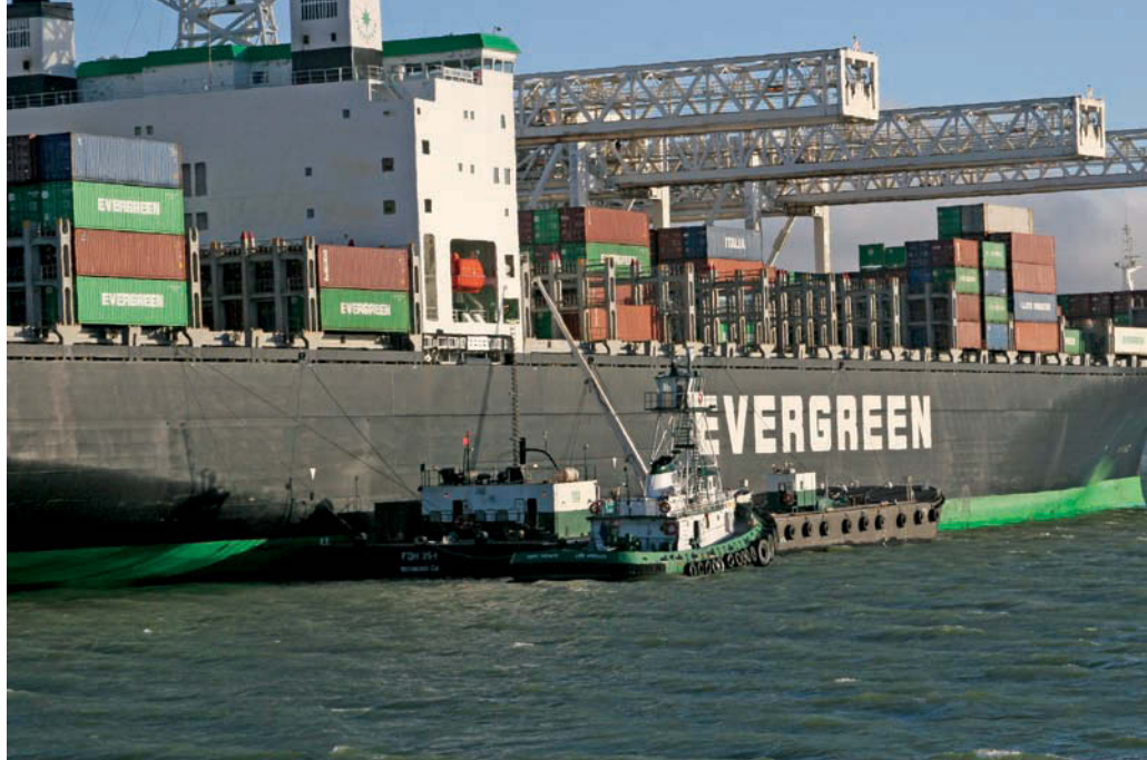
The Foss Tug Point Vicente and double-hull barge FDH 35-1 deliver bunker fuel to an Evergreen containership at the Port of Oakland. Bunkering is a major portion of Foss' business on the Bay
