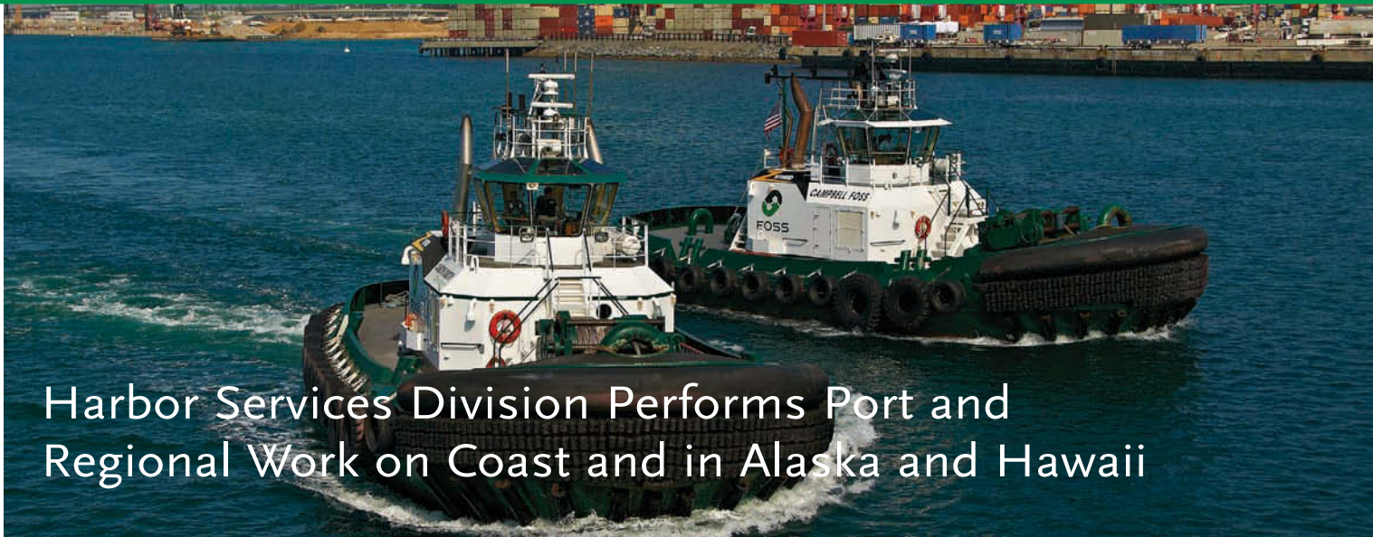
The Carolyn Dorothy , left, and Campbell Foss are hybrid powered tugs stationed in Long Beach.
