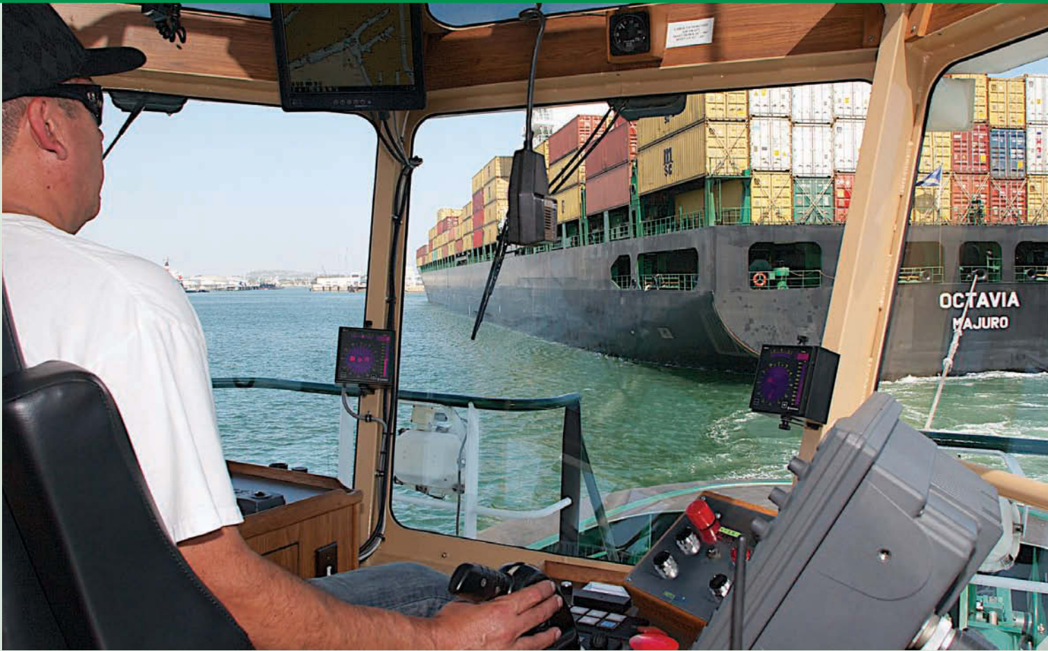
4. Engel uses the tug's power to turn the ship, preparing to back it into its berth at Terminal A.
