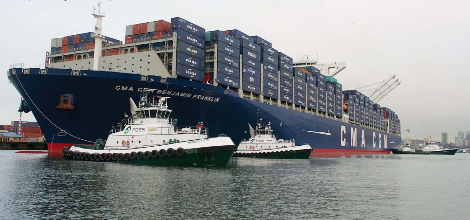
The tug Wedell Foss was in the lead and the Lindsey Foss was on the stern, moving the Benjamin Franklin past downtown Seattle and into the port's East Channel toward Terminal 18. The Henry Foss and Marshall Foss also participated in the assist. Aerial photo by Don Wilson , Port of Seattle.
