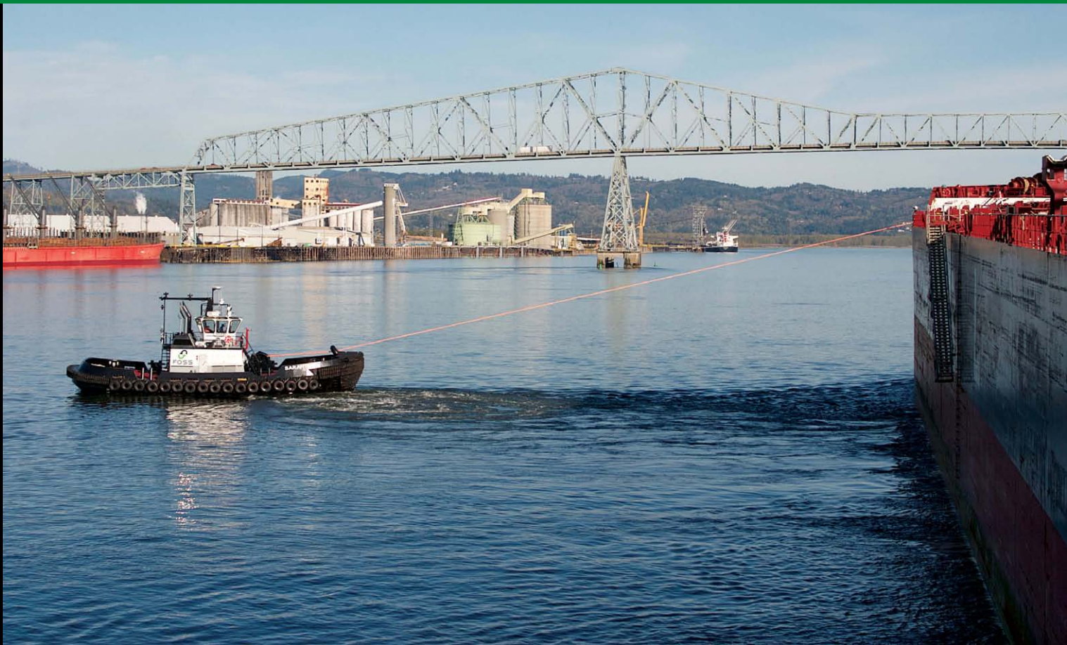
▲ 4. Above: The Sarah pulls the ship's bow away from the dock, enabling it to catch the current and spin downriver.
