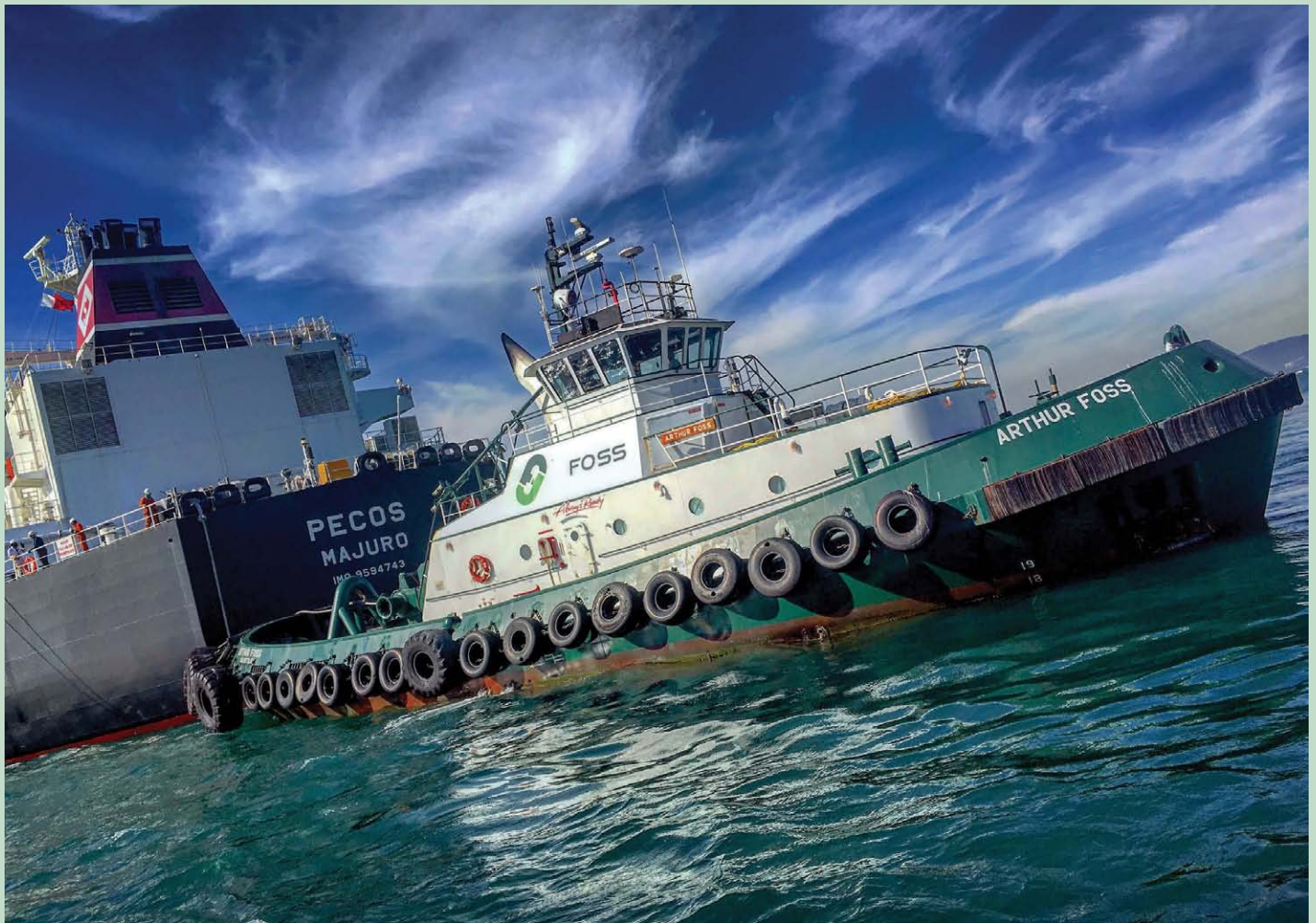
UNDER A SWIRLING SOCAL SKY Deckhand Nick Bristol caught this photo of the tractor tug Arthur Foss assisting the crude oil tanker Pecos into the El Segundo Moorings Berth 4 recently. The tanker is 898 feet in length and is listed at 158,465 deadweight tons.
