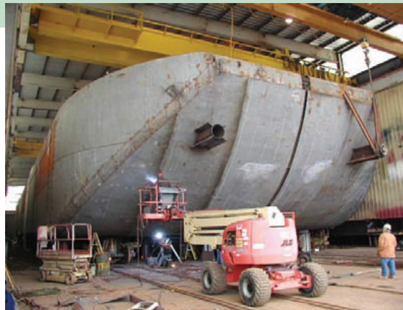
This recent photo shows one of two double-hull barges currently under construction for Foss at Orange Shipbuilding.
